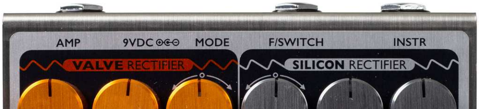
Rear connections. Right to left: Instrument input; External Footswitch; Power; Output
