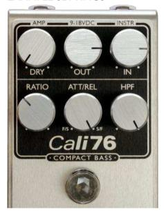
Percussive, lively & fat. A slow attack time allows the compressor to accentuate the initial transient of any given note. Fast release allows the compressor to fully recover between notes, so that every phrase and chord will take on a percussive quality. Low ratio keeps compression artefacts / distortion to a minimum. High HPF results in fattened low bass frequencies.
