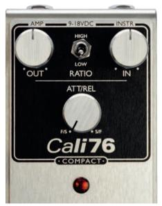
Dynamic control. A fast attack time allows the compressor to catch transients early on. A slow release time stops the compressor from pumping, making gain reduction mucg more stable. Compression is natural sounding and playing dynamics are evened out between melody and chordal passages.
