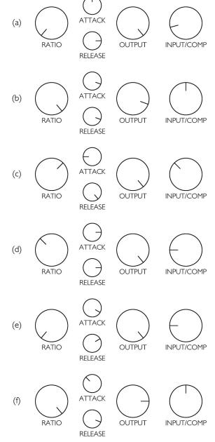
Figure 4: Useful Settings: (a) vocals - subtle compression; (b) vocals - limiting; (c) acoustic guitar / piano; (d) bass; (e) drums - subtle compression (famous Dr.Pepper Setting); (f) drums - "pumping" hard compression. Note: All source signals normalised to -10dBV.
