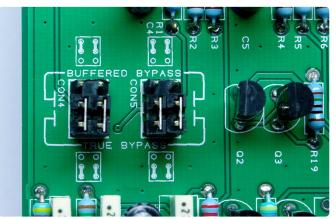
Figure 2: J4, J5, J6, J7: Bypass Jumper-Connectors.
