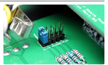
Figure 3: Input sensitivity jumpers on Cali76TX.
