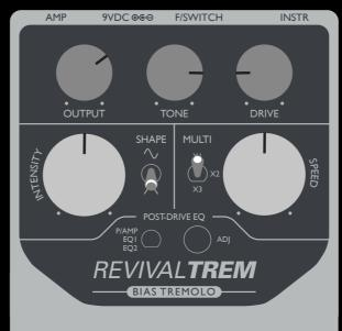
The RevivalTREM cleans up just like a valve amp. To achieve a clean tremolo sound, dial back the GAIN control and compensate for any volume loss with the OUTPUT control. The \( \simes\) wave shape is most pronounced at slow tremolo speeds. Switch to the X3 MULTI position for a fast and choppy '60s feel.
