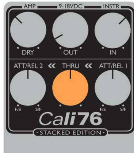
**Always on.** Compressors can fight your dynamics - cranking up the dry knob gives you back dynamic control. Known as "parallel compression", this is an established studio recording technique that allows you to combine the tone thickening, increased sensitivity and sustain of the compressed signal with the natural dynamic expression in your playing. So good you won't want to switch it off!
