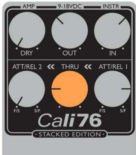
**Stacked compressors.** Each compressor is set up for a different task; the first gently evening out dynamics and the second clamping down and limiting peaks. A classic studio technique. Adjust the Thru control to your instrument and playing style. Start with the Thru control anti-clockwise and turn it clockwise until loud chords are limited causing the left VU meter to glow brightly.
