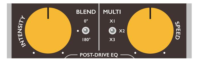
**SPEED:** Turn clockwise to increase the rate of the modulation effect. The range of the SPEED control is set by the three-position MULTI switch.
