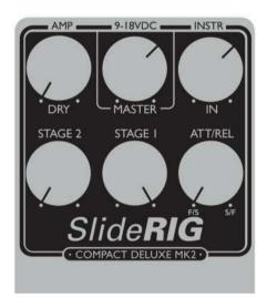
Conventional compression. Here we have the blend dial set anti-clockwise for a single stage of compression with a fast attack to catch peaks and a slow release to avoid pumping. Basically the same signal path as our Cali76 pedal. Great as a general guitar compressor, to smooth out dynamics and make your guitar feel a little more sensitive and alive. Ultra versatile.
