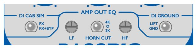
The post-drive AMP OUT EQ ensures compatibility with a wide range of amps and cabs. Instead of compromising your amp's tone controls to suit the BASSRIG, set your amp for your preferred clean sound then use the EQ controls to adjust the pedal's output accordingly (see tables on page 8).
