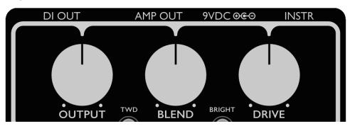
**9VDC:** Connect a 9VDC 2.1mm centre-negative mains power adaptor (minimum 150mA).
