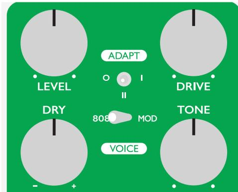
**ADAPT SWITCH:** This enables the Adaptive circuitry, allowing the pedal's mid-forward voicing to gradually fade away as the pedal cleans up. This gives you classic TS808 tone with your guitar cranked but reveals the full spectrum of your clean tone as you roll back the volume knob.
