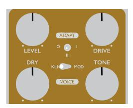
**ADAPT SWITCH:** This enables the Adaptive Circuitry, allowing the pedal's mid-forward voicing to gradually fade away as the pedal cleans up. This gives you classic Klon® tone with your guitar cranked but reveals the full spectrum of your clean tone as you roll back the volume knob.
