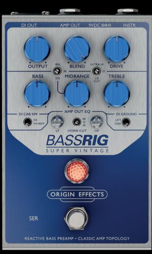
FOR THE FULL OWNER'S MANUAL VISIT WWW.ORIGINEFFECTS.COM **MIDRANGE** - This control can cut or boost mids at three different frequencies. Cutting the lower frequencies, especially with clean sounds, will result in a clear, scooped tone. Boosting the higher mids with an overdriven sound can create some fierce, howling rock distortion.
