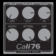
**PERCUSSIVE, LIVELY & FAT:** Using a slower attack time allows the compressor to accentuate the start of any note. Using a fast release allows the compressor to recover between notes so that phrases sound more percussive.
