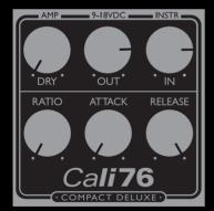
**PERCUSSIVE & LIVELY:** Using a slower attack time allows the compressor to accentuate the start of any note. Using a fast release allows the compressor to recover between notes so that phrases sound more percussive.
