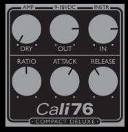
**DYNAMIC CONTROL:** A fast attack time allows the compressor to catch transients early on. A slow release stops the compressor from pumping. These settings sound natural and balance playing dynamics.
