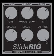
**DUAL-STAGE COMPRESSION:** This setting combines Stages 1&2 in series for maximum compression and sensitivity. Turn the ATT/REL control clockwise to preserve some attack in this classic, clean slide tone.
