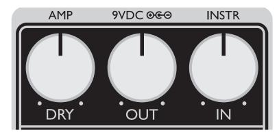
**9VDC:** Connect a 9VDC 2.1 mm centre-negative mains power adaptor (minimum 200mA). Voltage is increased internally for additional headroom.
